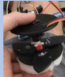
Figure 15: Air Brake Internal SetUp
