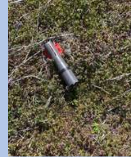
Figure 17: Wreckage of Launch Vehicle Resulting from Faulty Parachute Mechanism
